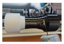
Figure 1. Filament winding of carbon– fibre on rocket nozzle form.
