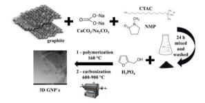
Fig. 1. The concept of the synthesis
